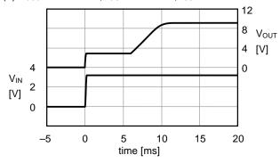
(3)  $f_{OSC} = 700 \text{ kHz}$ ,  $I_{OUT} = 0 \text{ mA}$ ,  $t_{SS} = 10 \text{ ms}$
