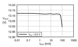
(2)  $f_{OSC} = 700 \text{ kHz}$ , MaxDuty = 77 % ( $R_{OSC} = 200 \text{ k}\Omega$ ,  $R_{Duty} = 300 \text{ k}\Omega$ )
