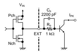
Figure 11 External Transistor Periphery
