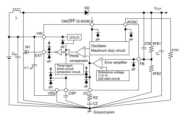
Figure 16 Standard Circuit (S-8338 Series)
