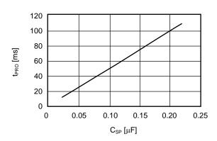
Figure 14 C<sub>SP</sub> vs. t<sub>PRO</sub>
