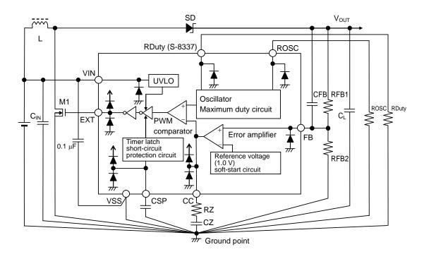
Figure 15 Standard Circuit (S-8337 Series)
