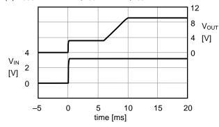
(2)  $f_{OSC} = 1133 \text{ kHz}$ ,  $I_{OUT} = 100 \text{ mA}$ ,  $t_{SS} = 10 \text{ ms}$
