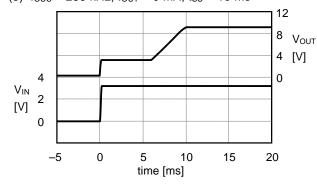
(6)  $f_{OSC} = 286 \text{ kHz}$ ,  $I_{OUT} = 100 \text{ mA}$ ,  $t_{SS} = 10 \text{ ms}$
