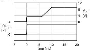
(4)  $f_{OSC} = 700 \text{ kHz}$ ,  $I_{OUT} = 100 \text{ mA}$ ,  $t_{SS} = 10 \text{ ms}$
